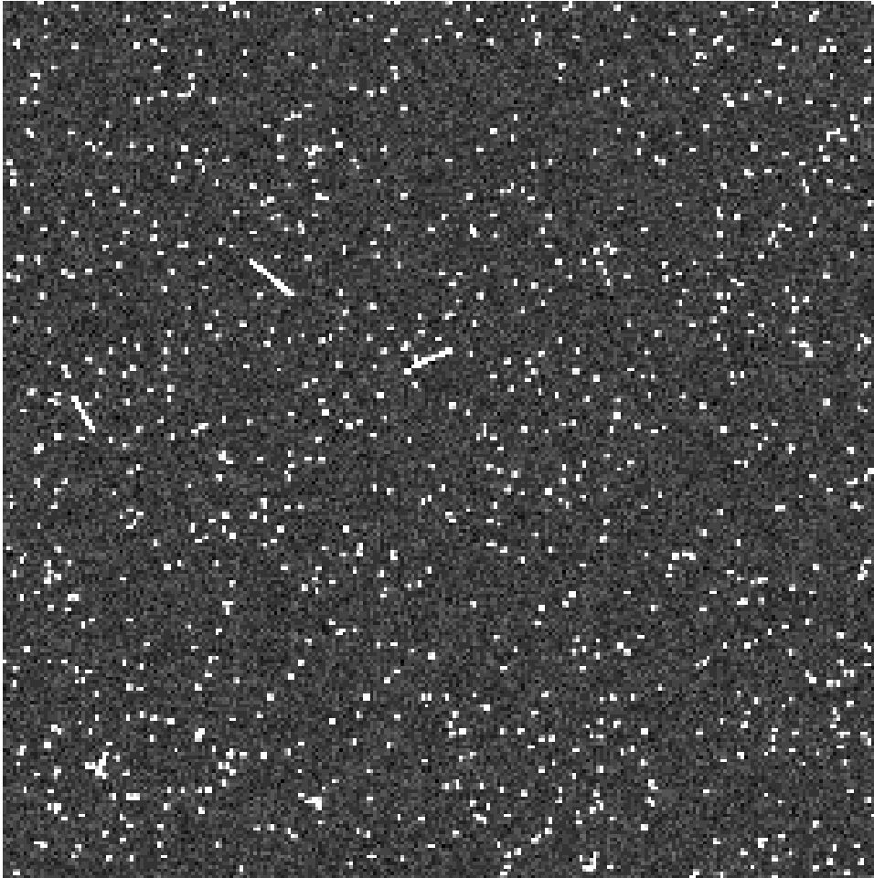
Figure 4.9: Example of a simulated back-illuminated CCD frame, containing 1000 1 keV photon events and 10 particle events
