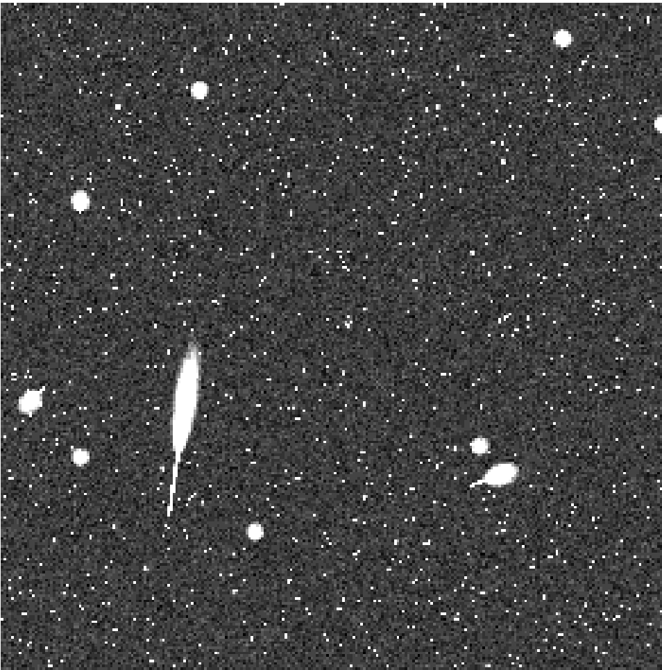
Figure 4.10: Example of a simulated front-illuminated CCD frame, containing 1000 1 keV photon events and 10 particle events
